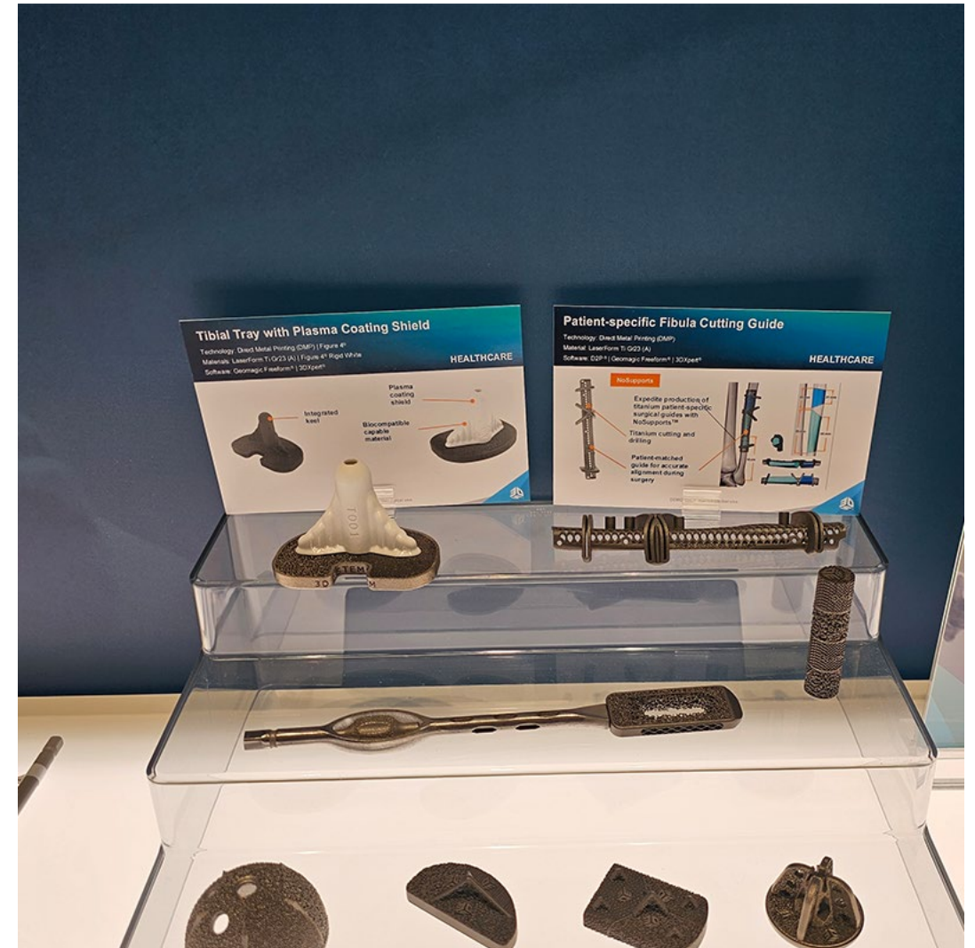
Tibial Tray with Plasma Coating Shield & Patient-specific Fibula Cutting guide. Menetelmä: DMP, Materiaali: LaserForm Ti Gr23 (A), Valmistaja: 3D Systems
