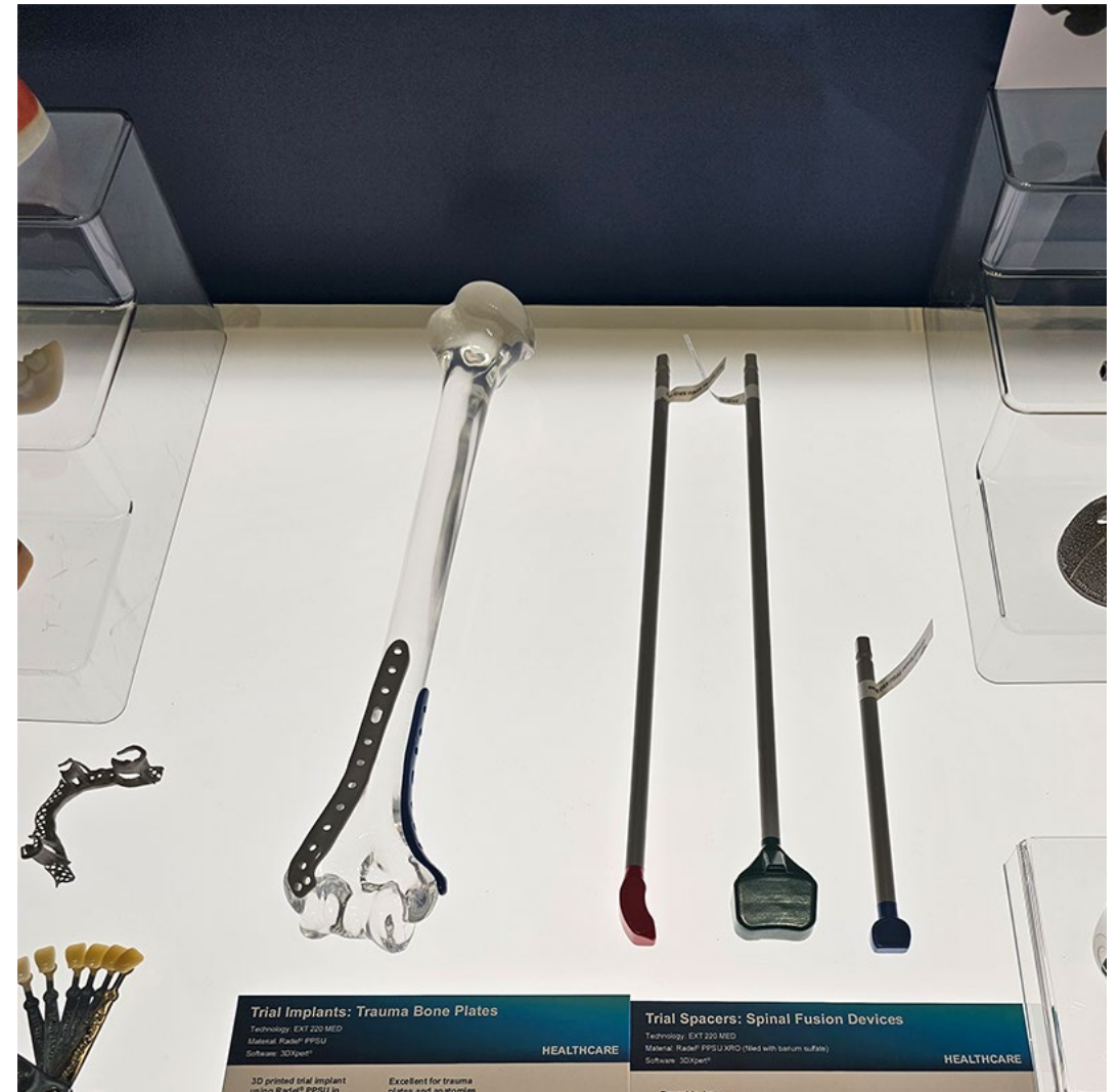
Trial implants & spacers: Trauma bone plates & Spinal Fusion Devices. Materiaali: Radel PPSU & Radel PPSU XRO (filled with barium sulfate). Valmistaja: 3D Systems
