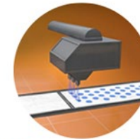
THEN, THE BINDING FLUID IS APPLIED, CAUSING THE PARTICLES TO BIND TOGETHER
